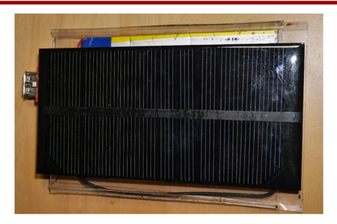
A solar panel charges a battery which provides power to charge a cell phone. But the cell phone requires 5V to charge and the battery only provides 3.7V, so we'll also need a voltage converter circuit.
