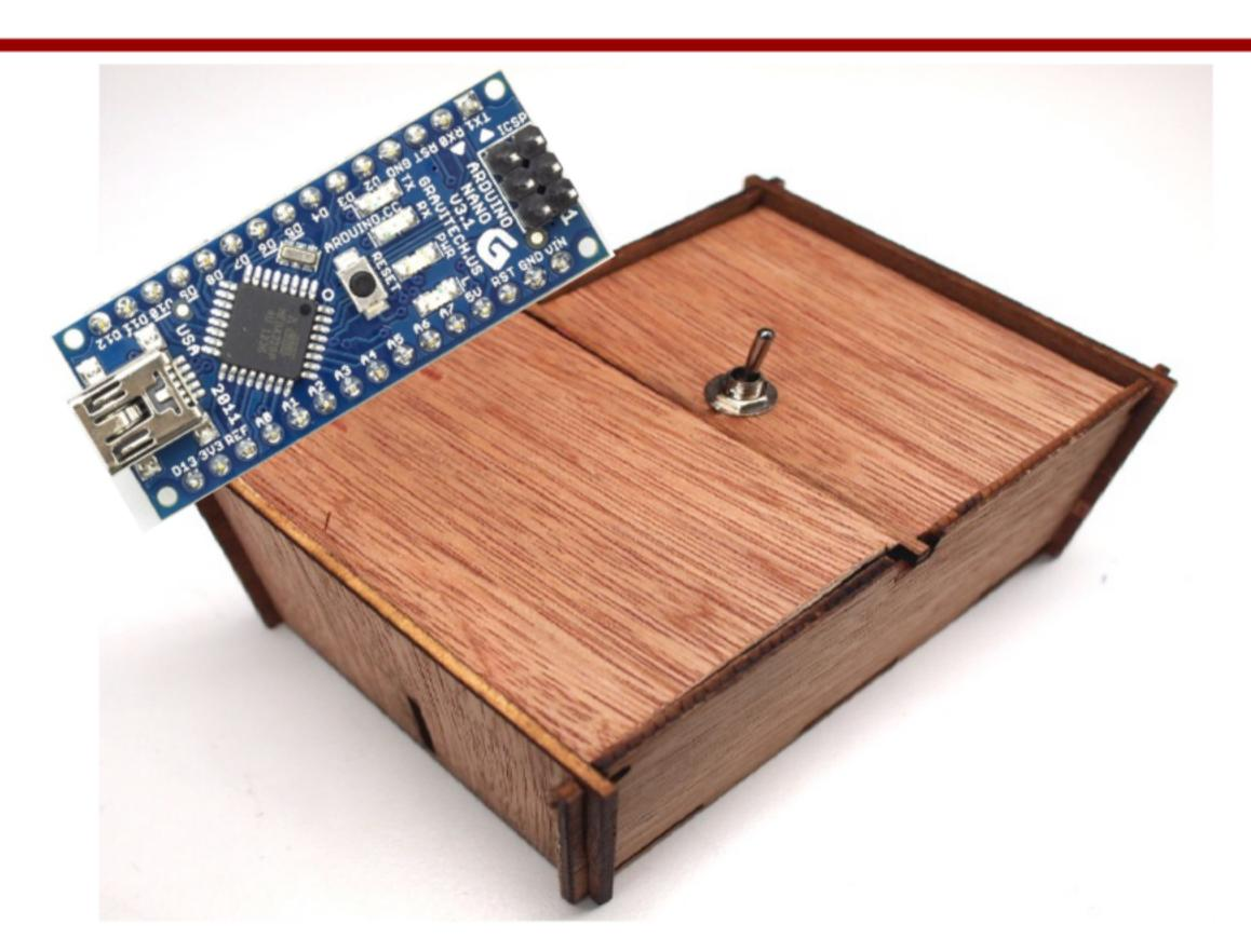
In this lab you'll assemble a "useless box" like the one featured in Make Magazine & on YouTube. When the switch on the box is flipped "on", a finger comes out of the box and turns the switch "off".
