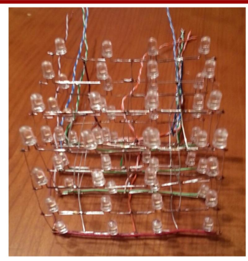
An LED cube is a 3D shape made entirely of light emitting diodes. The LED cube is wired to a computer (Arduino) which controls individual LEDs to display interesting patterns.
