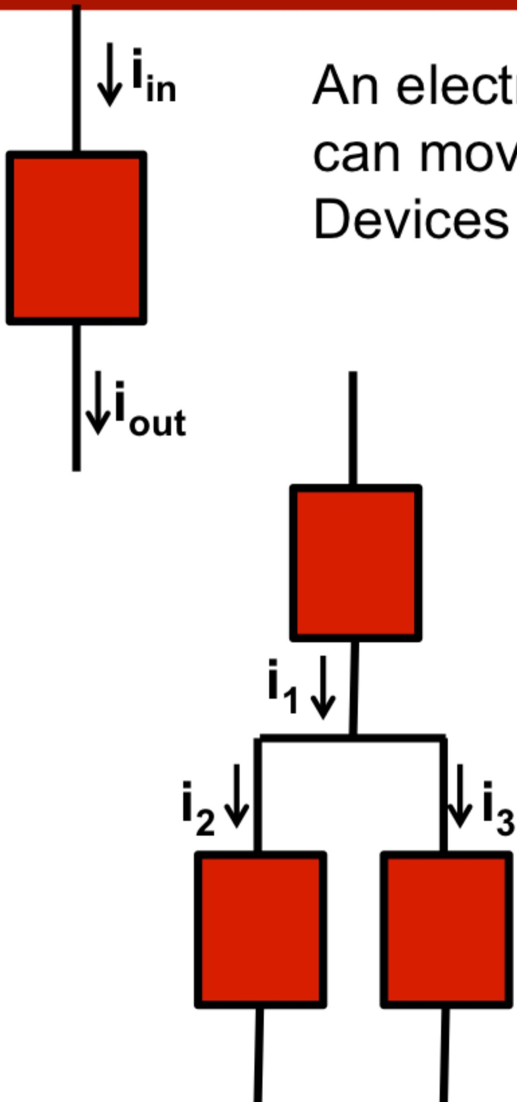
An electrical device is an object that charge (electrons) can move through, so current can flow through it. Devices are neutral (zero charge), so that
