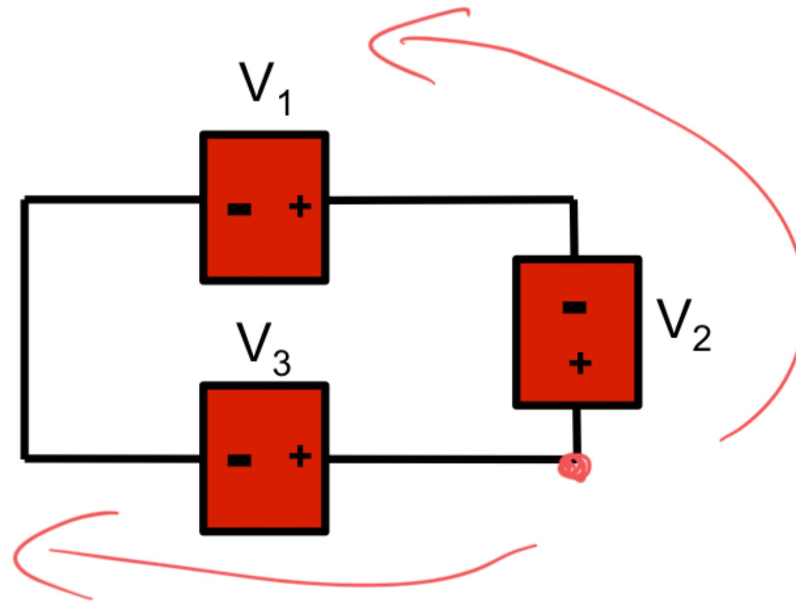
Kirchhoff's Voltage Law (KVL) states that the algebraic sum of the voltages around any closed path must be zero. So, for example,
