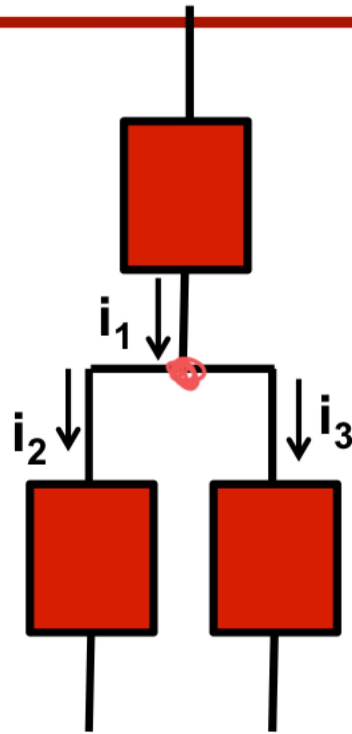
Kirchhoff's Current Law (KCL) states that the current flowing out of any node must equal the current flowing in. So, for example,
