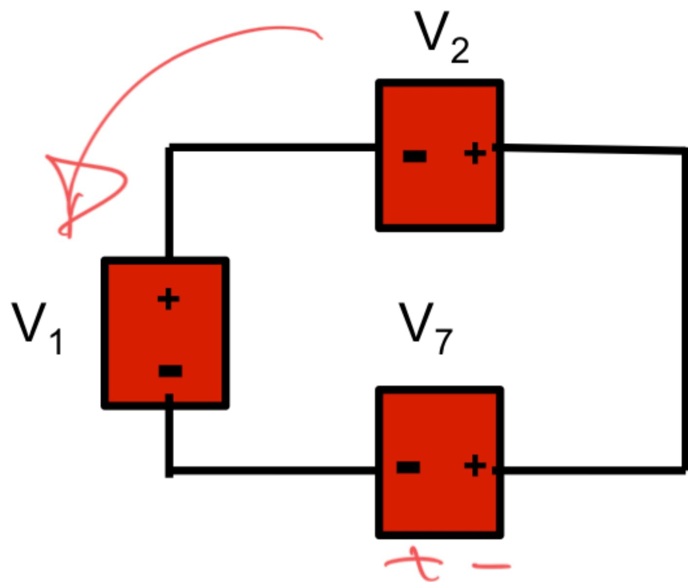
$$V_1 + V_2 - V_7 = 0$$
