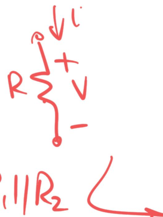
$$i_1 = \frac{V}{R_1} ; i_2 = \frac{V}{R_2}$$
