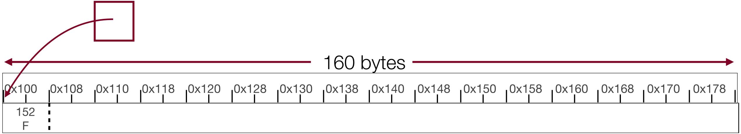
We use two blocks in the payload of the free block to point to the next and previous free blocks.
