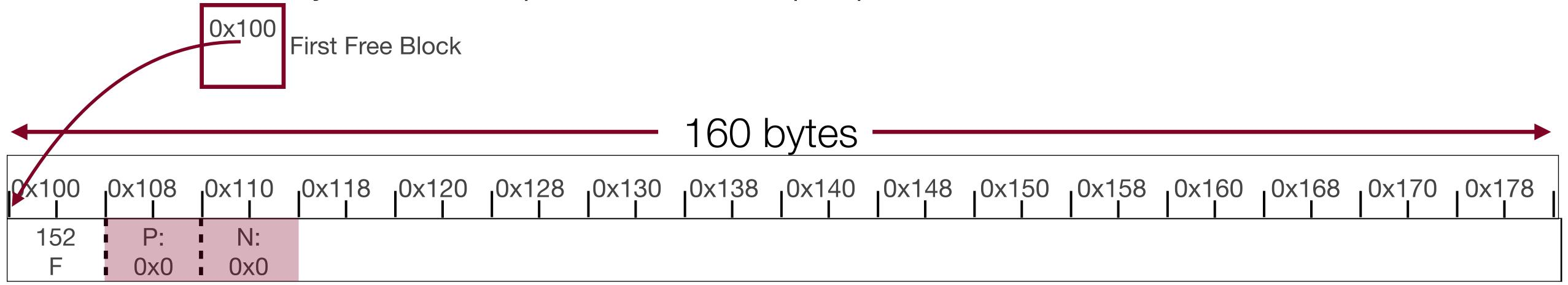
We use two blocks in the payload of the free block to point to the next and previous free blocks. In this case, there aren't any more free blocks, so they are **NULL** pointers.
