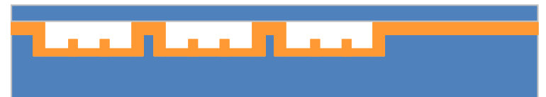
f) Silicon etch-back to form the membrane
