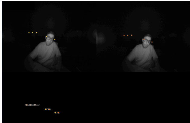
Figure 8. Bottom left corner show rectangles around corresponding markers yielding to epipolar constraint
