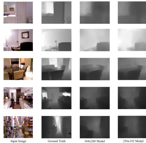
Figure 3. Comparison of depth maps after 3 epochs of training, with the U-Net model with a kernel size of 3 and the channel reduction filter in the up-projection layers, trained at 384 \times 288 and 256 \times 192 . These five images are randomly sampled from the test split of NYU-Depth V2.
