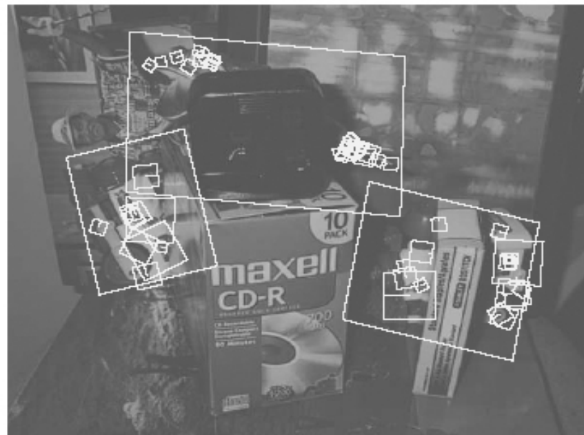
Figure 12: The training images for two objects are shown on the left. These can be recognized in a cluttered image with extensive occlusion, shown in the middle. The results of recognition are shown on the right. A parallelogram is drawn around each recognized object showing the boundaries of the original training image under the affine transformation solved for during recognition. Smaller squares indicate the keypoints that were used for recognition.
