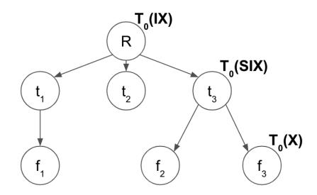
Suppose that this database is currently running only one transaction  $T_0$ . This transaction has already acquired the locks it needs as shown in the figure. For each of the other transactions below, indicate whether it can successfully acquire the locks it needs and run. If yes, provide the locks it acquires; otherwise explain the reason. *Note: Consider each transaction below separately, all based on the locks T<sub>0</sub> is holding at the start.*
