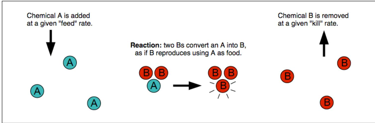
**Diffusion:** both chemicals diffuse so uneven concentrations spread out across the grid, but A diffuses faster than B.
