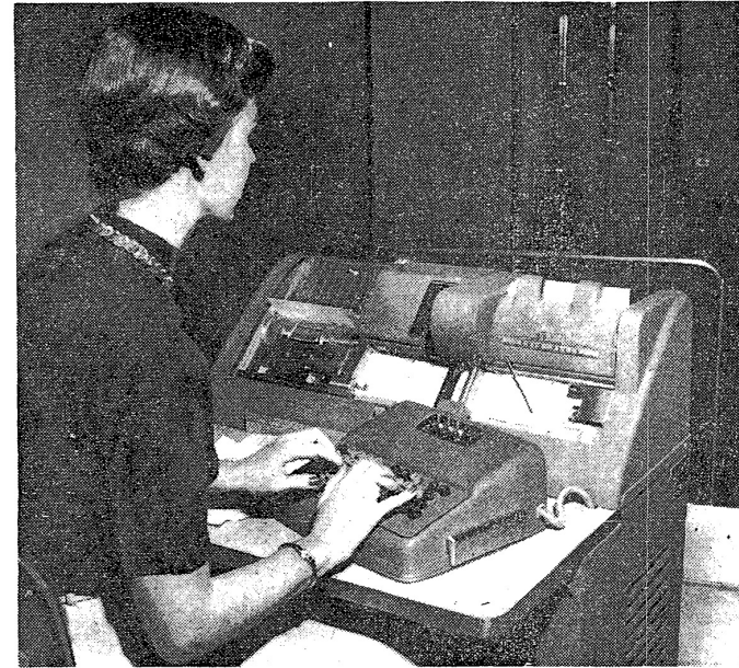
The New York Times An electronic calculator produced by the International Business Machines Corporation was demonstrated yesterday in a new role: translating Russian phrases into English. The device has a "vocabulary" of 250 Russian words and can be adapted to other languages. Miss Marilyn Folle "types" Russian phrases on I. B. M. punch cards that are fed into the machine.
