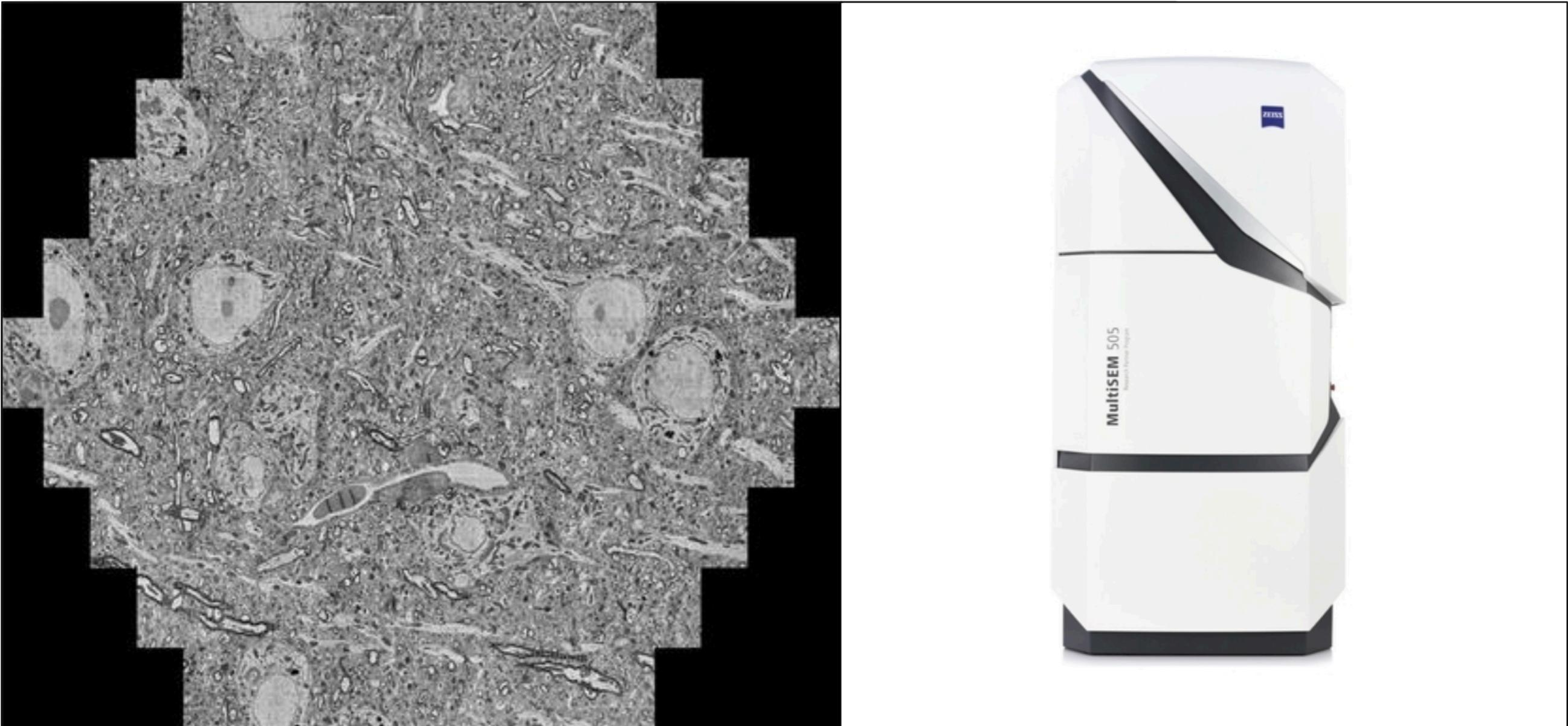
High throughput multi-beam EM imaging with up to 91 parallel beams operating at 2 terapixels per hour with 3.5 nm resolution or better
