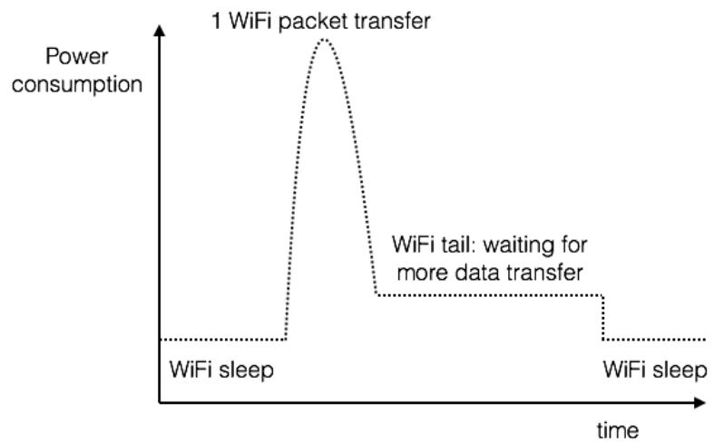
Instead of transmitting 1 WiFi packet each time, patch the packets and do bulk transmission to minimize the tail energy overhead.
