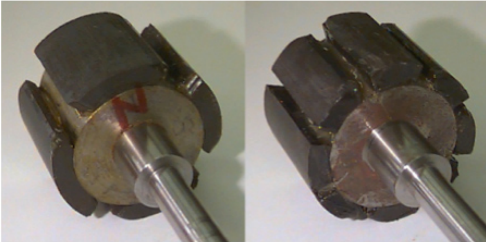
Figure 3: 4 pole and 8 pole – Permanent magnet rotor
