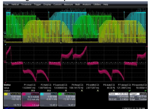
Figure 7: 6-Step Phase Current from Scope
