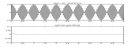
We can end up transmitting with a cosine, and receiving with a sine. These are orthogonal, and we get nothing!
