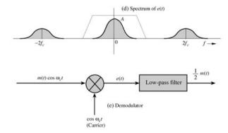
The low pass filter does not have to be very sharp. But it should be flat over the signal baseband.
