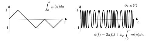
lacktriangle This results in exactly the same waveform given  $k_p$  is properly scaled.
