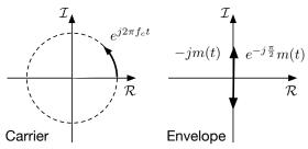
The envelope is now imaginary (the -j) or can be thought of as phase shifted by  $-\pi/2$ . This turns the cosine carrier into a sine.
