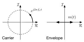
The message m(t) scales the amplitude of the carrier.
