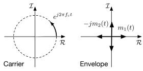
The magnitude of  $m_1(t) - jm_2(t)$  scales the amplitude of the carrier, and the angle adds to the phase of the carrier.
