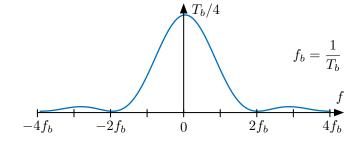
The bandwidth  $2f_b$  is  $4\times$  theoretical minimum of 2 bits/Hz/sec.
