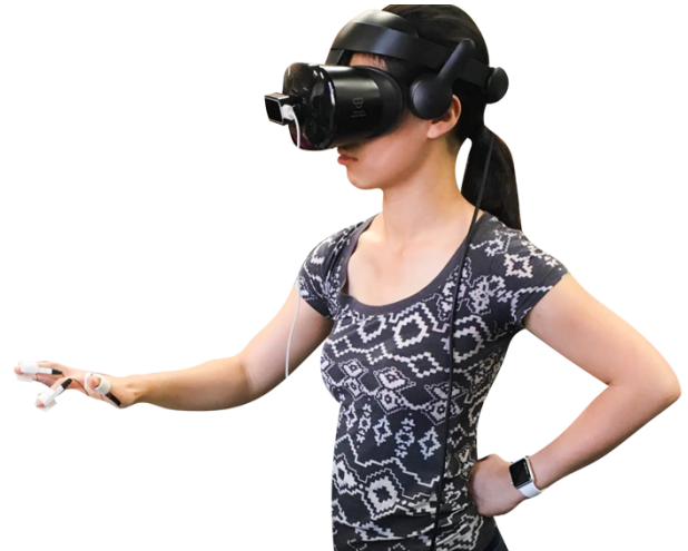
Figure 4. A subject performing the user study while wearing the Samsung HMD Odyssey VR headset with a Leap Motion hand tracker mounted on the front of the headset. Users wore the haptic devices on the thumb, index, and middle fingers of their dominant hand.
