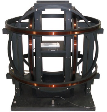
3 axis Helmholtz coil www.directvacuum.com
