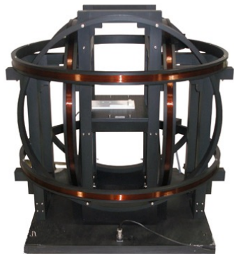
3 axis Helmholtz coil www.directvacuum.com
