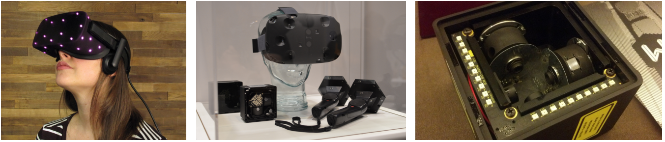
Figure 1: Examples of optical tracking in VR. Left: near-infrared (NIR) LEDs of the Oculus Rift recorded with a camera that is sensitive to NIR (image reproduced from ifixit.com). Center: HTC Vive headset and controllers with exposed photodiodes (image reproduced from roadtovr.com). Right: disassembled HTC Lighthouse base station showing two rotating drums that create horizontal and vertical laser sweeps as well as several LEDs that emit the sync pulse (image reproduced from roadtovr.com).
