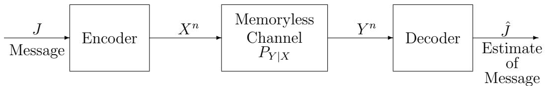
$J$  is a message uniformly distributed on  $\{1, 2, \dots, M\}$  passed into the system. The encoder maps message  $J$  onto its corresponding  $n$ -length codeword  $X^n$  from codebook  $c_n = \{X^n(1), X^n(2), \dots, X^n(M)\}$ . The encoded message is sent through a memoryless channel characterized by  $P_{Y|X}$ , and we receive  $Y^n$  as output.
