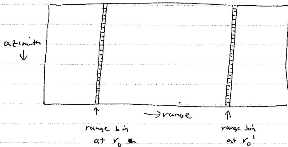
Two highlighted columns are shown. Each represents a sequence of complex azimuth samples which we can match-filter to derive azimuth resolution of  $\frac{\lambda}{2}$ . Our azimuth processing algorithm simply reads in samples down from each column in the matrix, applies the appropriate reference function, and outputs the correlation result.
