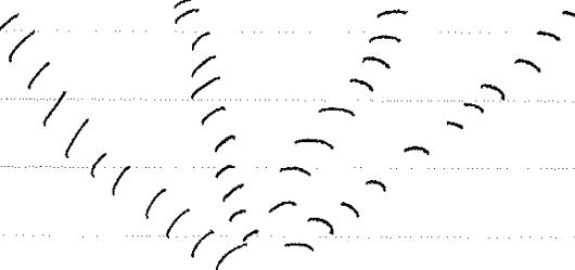
waves from object are summed in the processor after correction for platform motion
