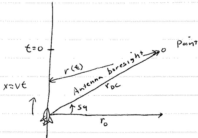
Let's let the subscript DC denote Doppler centroid, the time or location when the target point goes through the antenna boresight. Hence,  $r_{DC}$  is the range from the object to the radar at this instant, and so forth.
