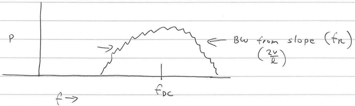
Note the time in the beam follows from the velocity and antenna length
