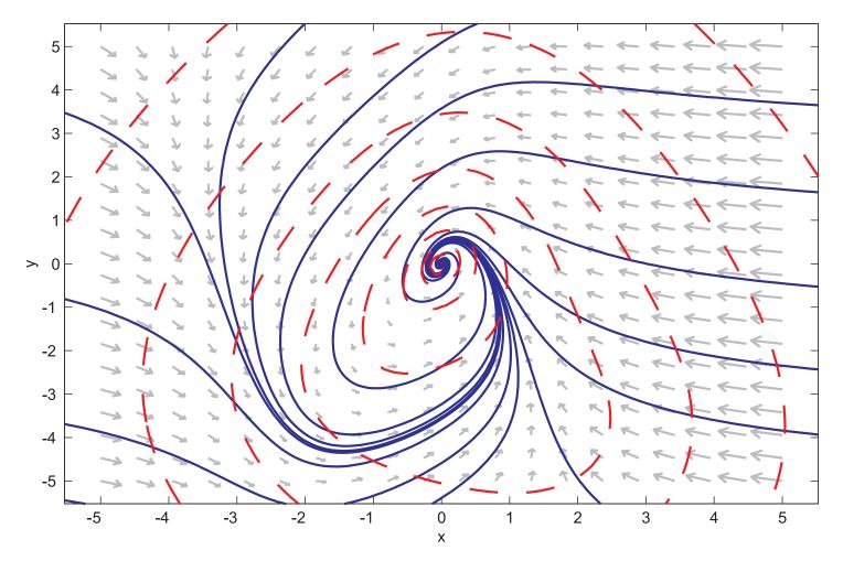
$V = 4.5819x^{2} - 1.5786xy + 1.7834y^{2} - 0.12739x^{3} + 2.5189x^{2}y - 0.34069xy^{2} + 0.61188y^{3} + 0.47537x^{4} - 0.052424x^{3}y + 0.44289x^{2}y^{2} + 0.0000018868xy^{3} + 0.090723y^{4}$
