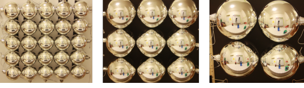
Figure 2. Spherical mirrors arranged in grids (2in diameter spherical mirrors arranged in a 5 \times 5 grid, 3\frac{1}{3} in diameter spherical mirrors arranged in 3 \times 3 grid and 5in diameter spherical mirrors arranged in 2 \times 2 grid)
