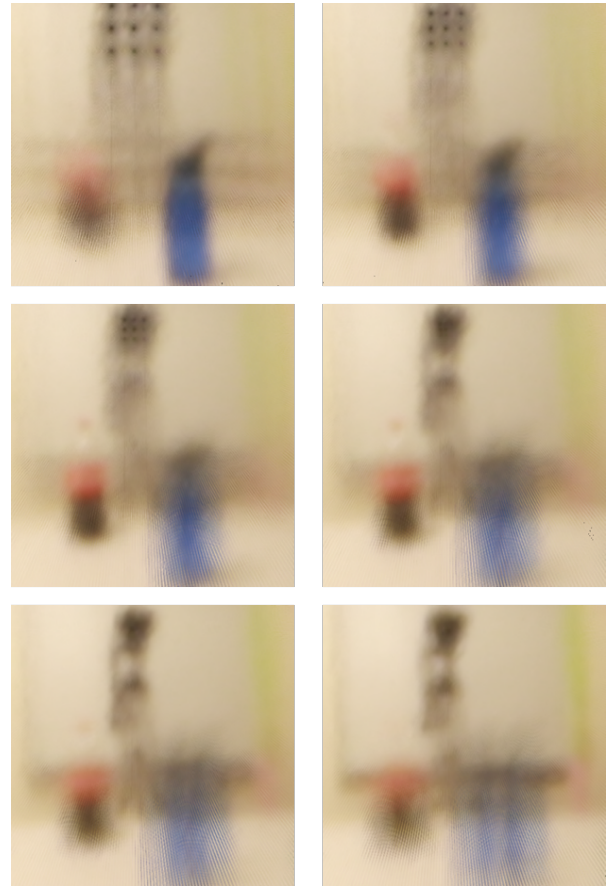
Figure 7. Refocusing using the 3 \times 3 light field showing the focal plane swept from close to far as you move down in the row or across columns.
