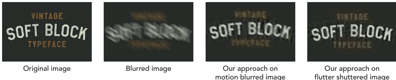
Figure 1: Using our method with images that are flutter shuttered results in clearer and more readable text when compared to images that are captured using a single exposure.
