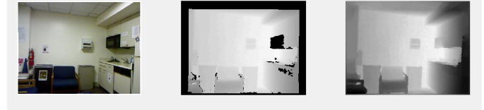
Figure 3: 1) raw image 2) depth output 3) depth output after post processing
