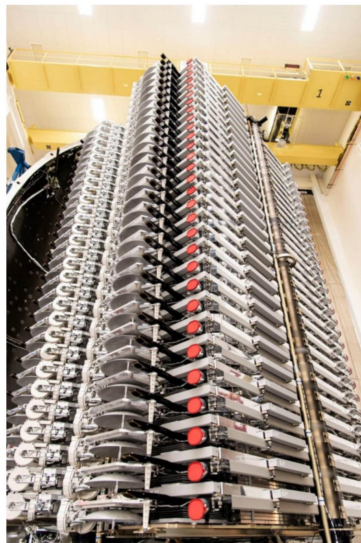
Fig. 1. A stack of 60 Starlink satellites prepared for launch. A Star Tracker camera, with red lens cover, is visible on each.
