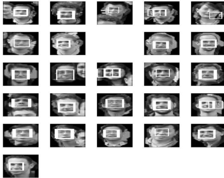
Figure 11: Output of our MRC Algorithm. Note the non-faces from Figure 10 have been removed, but nothing else has been. This is perfect detection.
