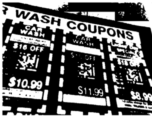
Figure 3: Binary version of input image after application of a three channel local threshold
