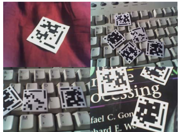
Figure 12: Four examples of test images that have multiple visual code markers at various projections. Some of the markers are not fully encapsulated by the image, and these markers were all successfully rejected as false positives
