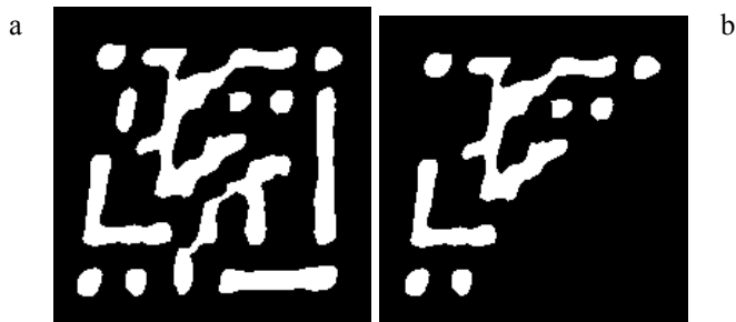
Fig 8. (a) shows Fig 7 converted to black and white using local image mean. (b) right shows the remaining patches of Fig 7a after selecting only regions with low eccentricity. Refined bounding point estimates are derived as the centers of the white regions closest to the three non-guide bars corners of the image.
