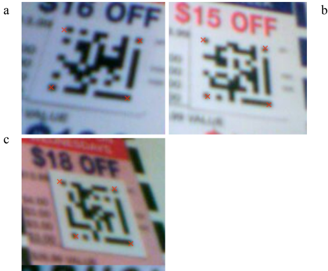
Fig 6. Red “x”s mark the preliminary estimates of the locations of the four bounding points for each valid visual code in Fig. 5 using the size and orientation of the guide bars only for prediction.
