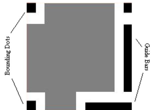
Fig 1. The visual code pattern to be detected. Black and white dots indicate fixed values on the pattern while gray dots indicate data bits that can be either 0 or 1.
