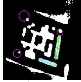
Fig. 6 (From training_6 image) A set of marker with two ellipses(green one is long GB and blue one is short GB) and corresponding three CEs with its search range symbolized as corresponding radius in each circle(in pink circles).
