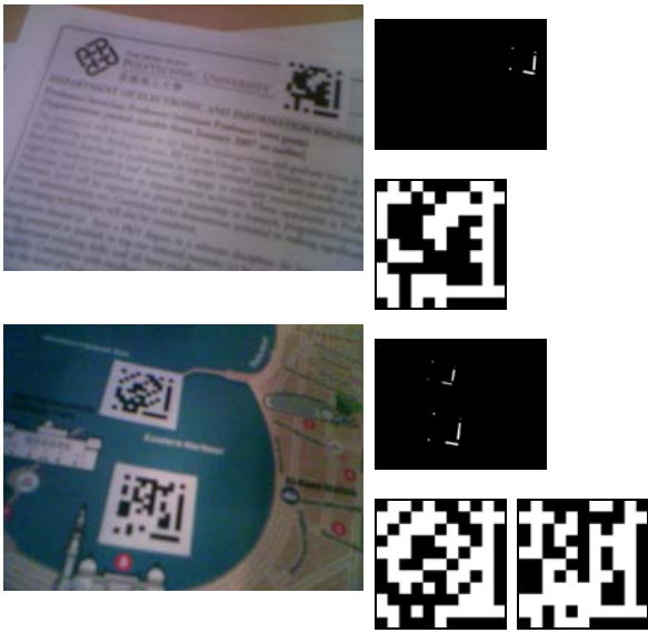
Fig. 10. Results of marker detection on training images.
