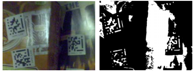
Fig. 9 Bad thresholding. The right marker is partly covered by sharp shadow. Thus, part of the marker is likely to be binarized to black and results in bad thresholding.
