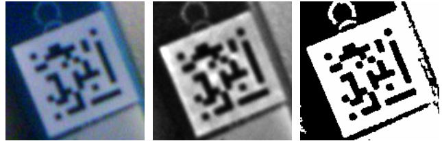
Fig. 1. (Left) Sample Marker Image. (Middle) After noise reduction and relative contrast enhancement. Light regions surrounded by dark regions have become brighter. The result is most apparent when comparing two markers within a non-uniformly lit image. (Right) After extreme sharpening and conversion to black and white. Images are shown at 50%.
