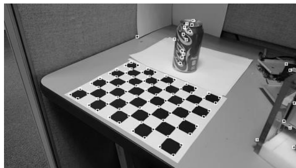
Figure-1: The image illustrates the original image in grayscale with the corners produced by the Harris corner detector.
