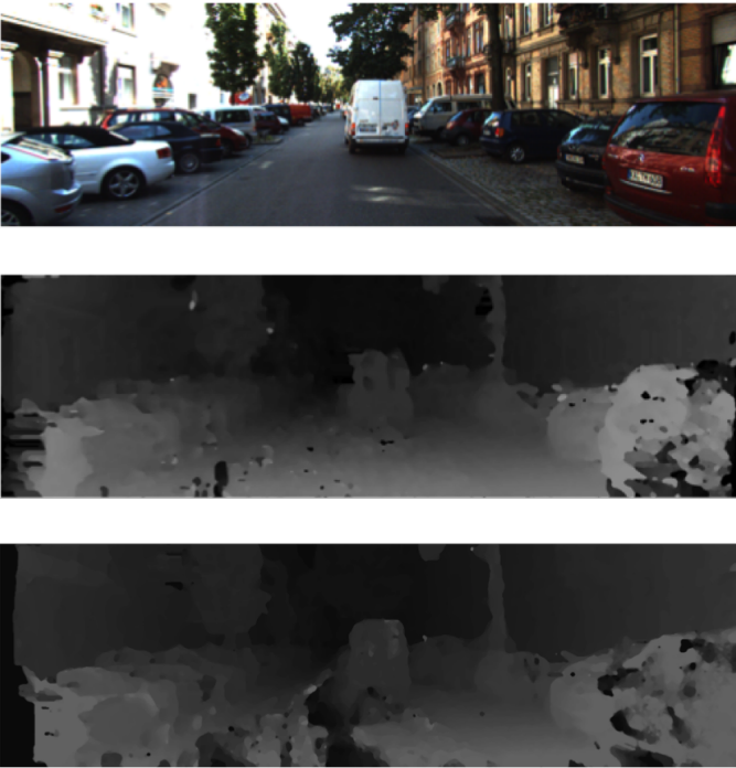
Fig. 10. (Top) the left image in the stereo pair.(Middle) disparity map created with the convolutional neural network. (Bottom) disparity map created with 9 \times 9 subtractive method. Reflections through off the disparity measure.
