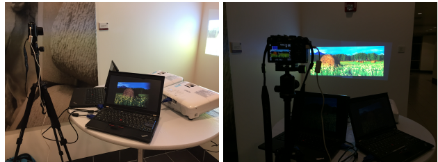
Figure 1. Setup includes a camera used for initial calibration, one or two projectors individually controlled by computer, and a screen.
