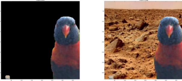
Fig. 4. Foreground mask applied to the center image from Fig. 1 and a new image superimposed onto the background.
