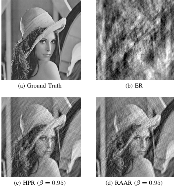
Fig. 3: A comparison of different projection algorithms. HPR gives the most accurate reconstruction with a normalized error of 0.1258.
