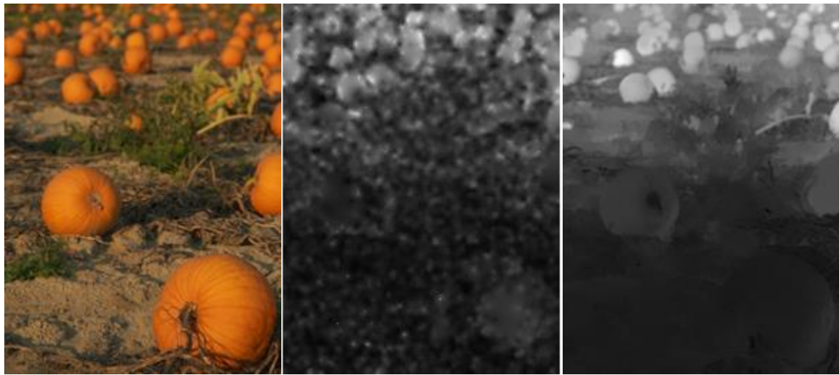
Figure 4: Obtain defocus map from input image a) by applying nearest neighbor method b) and matting laplacian c). Matting laplacian results in defocus map with good accuracy.
