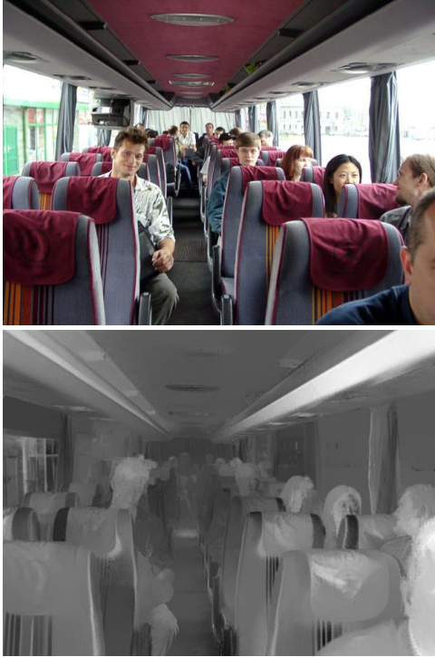
Figure D: a) Original image inside a length bus, b) Estimated full defocus map
