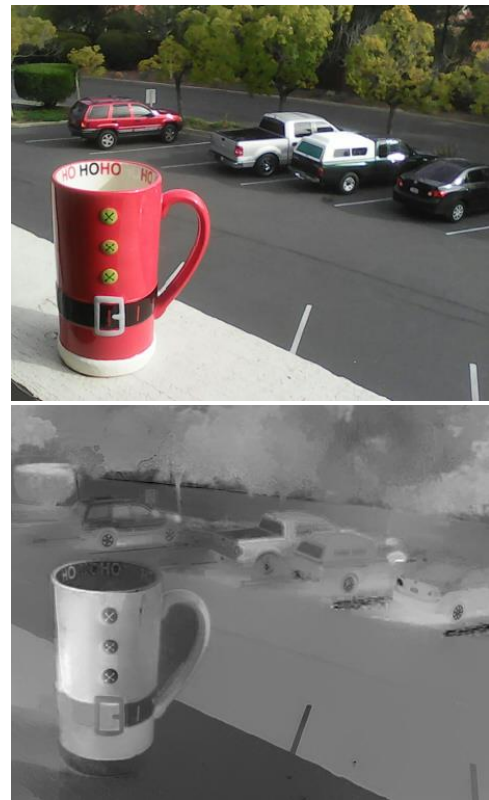
Figure C: a) Original image taken on Android camera, b) Estimated full defocus map
