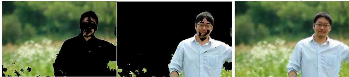
Figure 6: a) background based on segmentation; b) foreground based on segmentation; c) image with bokeh effect without face protection
