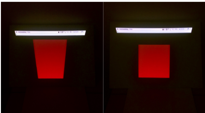
Comparison of original vs. corrected casted projection onto a posterboard with vertical incline with respect to the projector.
