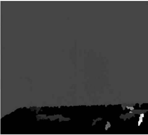
Figure 1: Unprocessed depth image of scene without object screen. The image is normalized by max value. The black region at the bottom of the image is the floor, and the remaining grey region is the back wall. As can be seen, the noise on the floor plane takes the form of blotches with large values of uniform depth.
