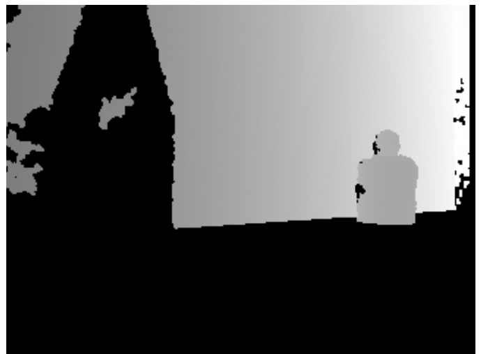
Example of depth image in which the object surface is occluded by two bottles. Object surface is placed with a horizontal incline with respect to the projector.
