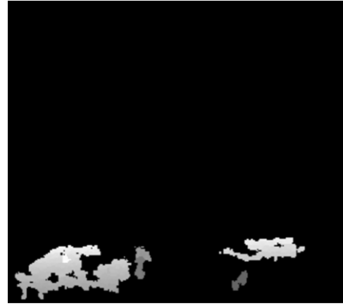
Figure 2: Depth image with background filtered out. Floor noise in this image is even greater than that seen in Figure 1.
