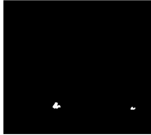
Figure 3: Depth image with background and floor thresholded out. Some noise still remains in some frames due to the depth values being too high at those locations.
