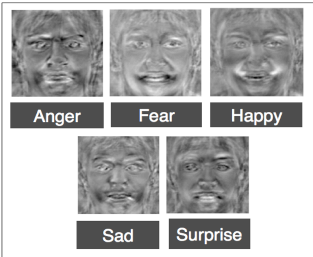
Fig. 2 Top eigenvectors reshaped to 100x100 images (Fisherfaces) after Fisher LDA for Anger, Fear, Happy, Sad and Surprise.
