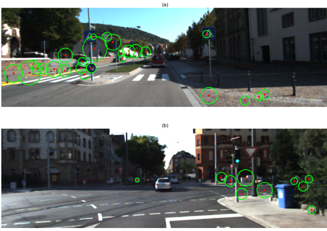
Fig. 5. Detecting round sign with Hough Circle Transform
