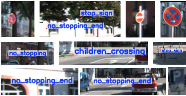
Fig. 10. Incorrect Detection or Unrecognized Signs
