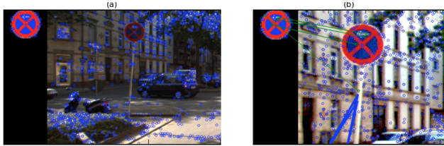
Fig. 11. Feature matching affected by illumination condition
