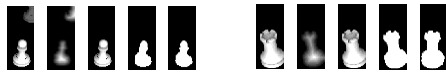
Fig. 2. Two sets of images showing extraction of piece (left to right) Test piece pawn; test piece rook; (sub images 1 to 4) small segment of image taken from the square which contained a piece; results of applying distance transform on image 1; segmented image after removal of noisy piece; mask of piece; mask of the piece after fixing the orientation
