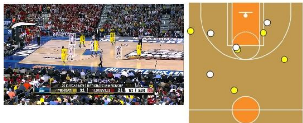
Fig. 7: Comparison between the players detected and the projected image in the court. As you can see the players match the position in the top-down court model.
