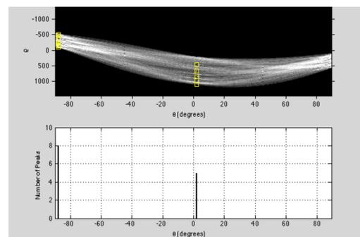
Fig. 2. Hough orientation histogram and peaks
