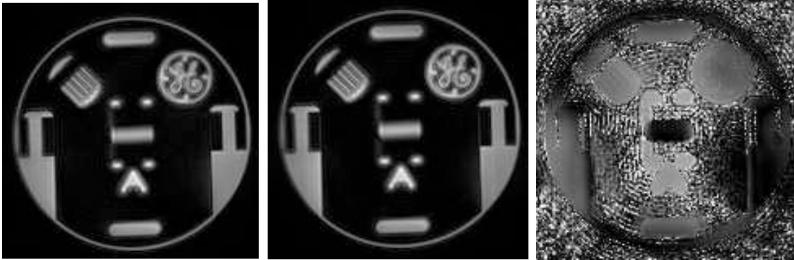
Figure 2: The two data sets look very similar. The first is at TE of 2.5 ms, and the second at 7.1 ms. The field map shows significant variations in frequency, which correlate well with the off-resonance blurring.
