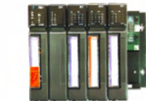
Programmable Logic Controllers (PLC)
