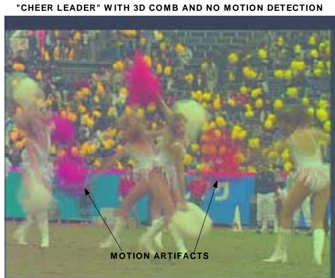
Figure 10 - Motion artifacts in 3D comb filtering
