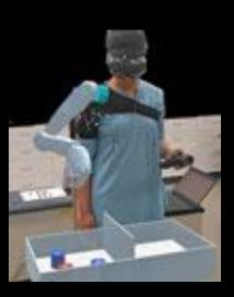
"At the ARM Lab, the **Intelligent Prosthetic Arm** (IPARM) project has built an immersive simulation platform to improve the control of powered prosthetic arms using computer vision and augmented reality."
